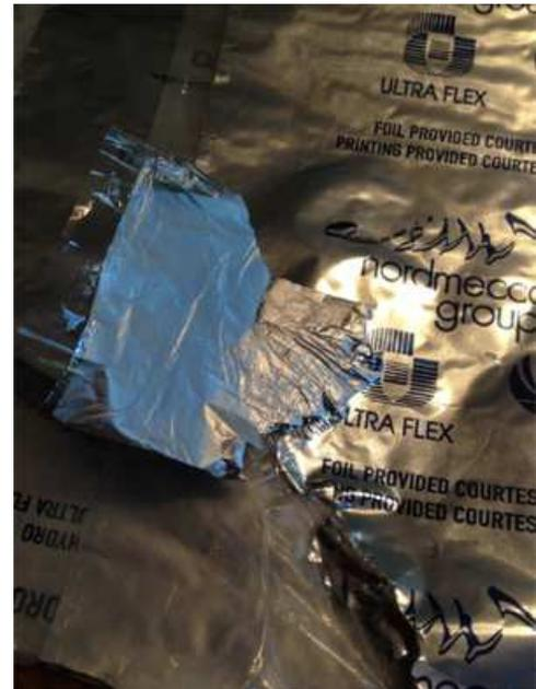
Foil adhesion was tested immediately after lamination, and daily thereafter, peeling an inch or so at a time. (Photo by Tom Bezignan)
